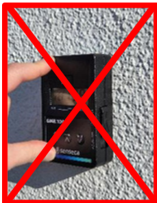
False: unsteady surface
